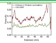
90° peel tests on graphite electrodes with chitosan binder show stronger adhesion to the copper collector compared to the CMC:SBR (2:1) benchmark, as evidenced by higher force values in the force-extension curve
