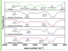
FTIR spectra of chitosan films solubilized in lactic acid show a decrease of carboxyl bands (1550 cm<sup>-1</sup>) and an increase of ester bands (1725 cm<sup>-1</sup>) with rising acid concentration. This indicates that part of the lactic acid remains bound in the polymer matrix, enhancing interfacial adhesion. So, 5 wt% lactic acid solution was selected for electrode fabrication.
